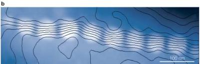
Figure 3 | Electron holography of a region of the magnetosome chain in *Magnetospirillum magnetotacticum*. a | Magnetosomes with the electron interference pattern. b | Magnetic field lines derived from the interference pattern superimposed on the positions of the magnetosomes. The confinement of the field lines within the magnetosomes is indicative of single magnetic domains and shows that the chain of magnetosomes acts as a single magnetic dipole.
